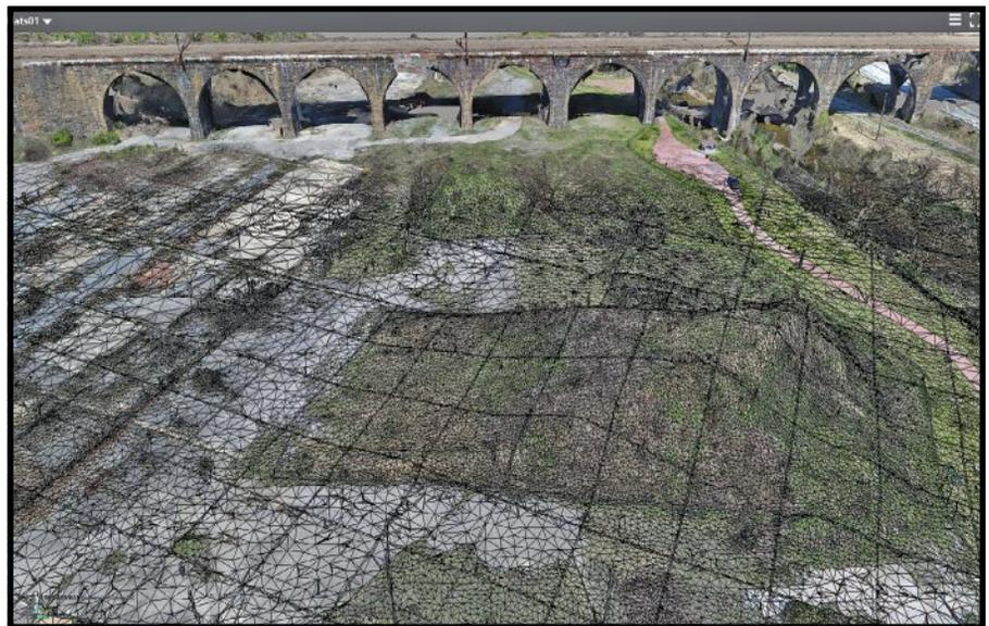
**Mass data capture solutions like mobile mapping systems, scanners, and UAS (top left) are producing data-rich point clouds and images that can be combined to yield full 3D models at any stage of the design/construct work flow, for example in ContextCapture (bottom). Updated 3D models can then be cloud-transferred to the site for machine control operations (top right).**
